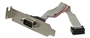
The PLATE9MLP 9pin Serial Male to 10pin Motherboard Header LP Slot Plate adds a DB9 serial port to the rear panel of small form factor/low profile computer, connecting to the host computer motherboard using an IDC10 connector.
